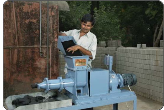
Making energy efficient briquettes
