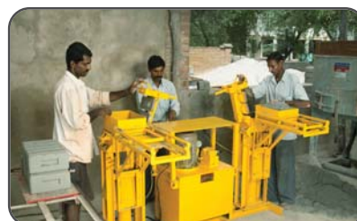
Compressed Blocks from Fly ash with TARA Balram
