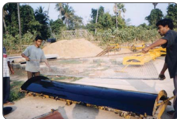
Making Roofing Channels using a Mechanized Ferrocement Production Table
