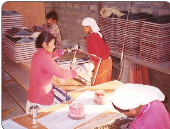
Micro Concrete Roofing Tiles - an alternate roofing technology
